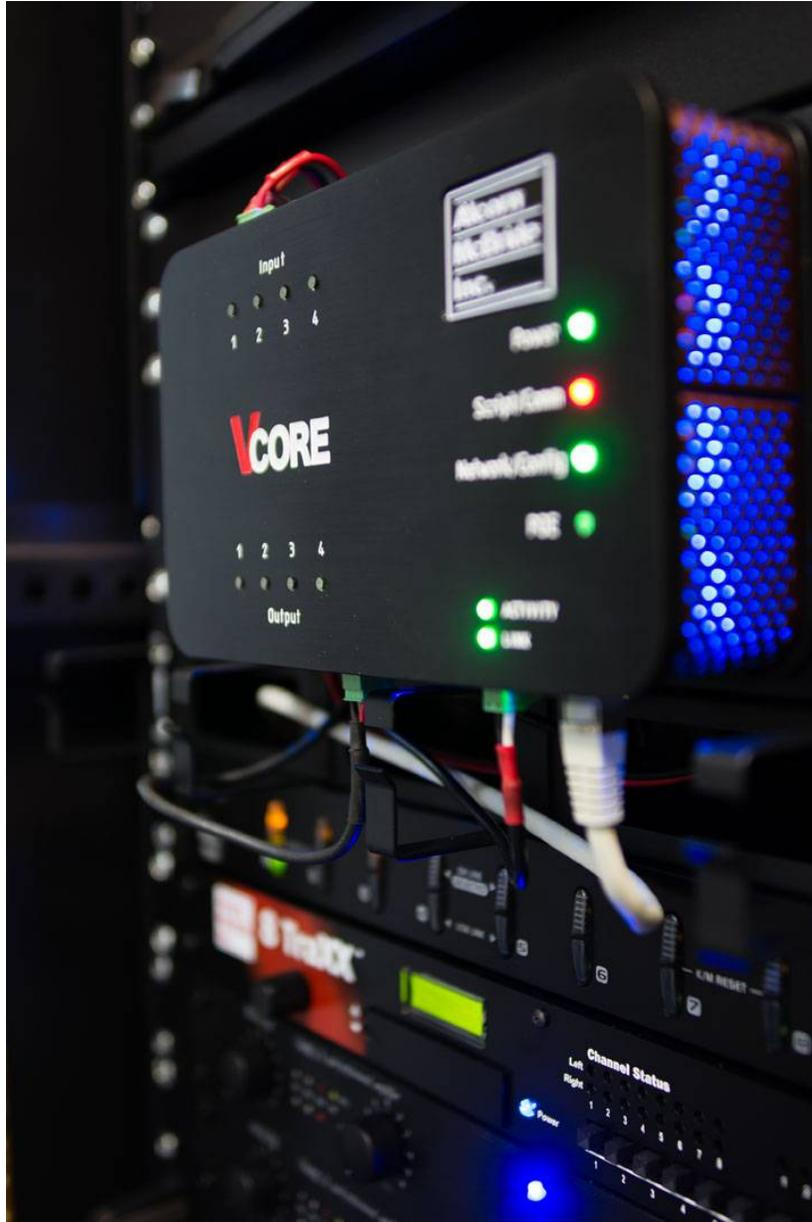
In addition, Alcorn McBride's 8TraXX multichannel audio player is used for background music and exhibit-specific sound effects throughout the museum. The 8TraXX stores clips in the MP3 format on CompactFlash media for a rugged, reliable and maintenance-free audio solution.
